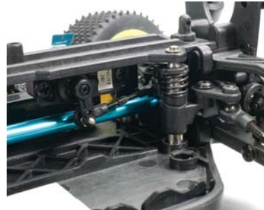
A buggy-style dual-bellcrank steering system points the tires in the direction you want the car to go. A built-in servo saver on the right bellcrank protects the servo. A steel turnbuckle links the bellcrank arm to the servo horn.
