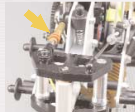
The silver spring acts as an additional front-end shock absorber, and the steering damper (arrowed) soaks up any bumps that might knock the front wheel off-course.
