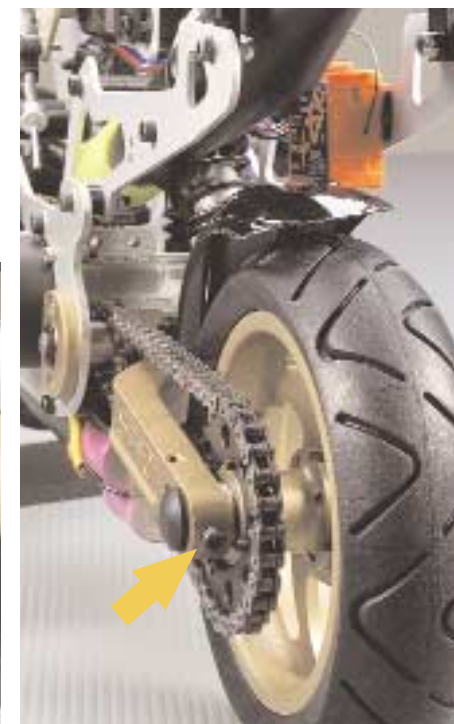
Right: the realistic-looking rear end features an authentic metal chain and a one-sided swing arm where the rear sprocket is mounted. The screw that's indicated by an arrow is used to adjust chain tension.
